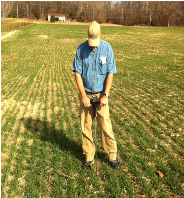
Figure 3. A soil penetrometer being used to diagnose soil compaction in a wheat field.
