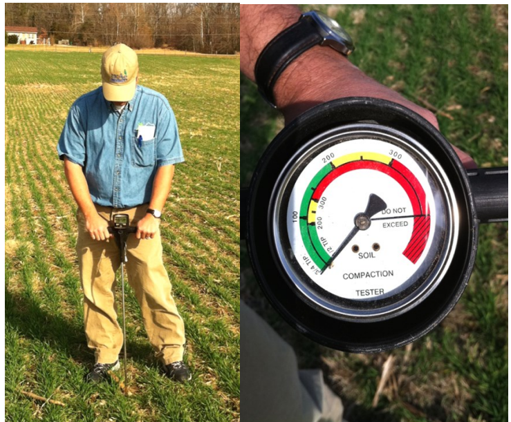
Figure 1. a) Using a soil penetrometer to determine the depth and degree of soil compaction by b) following the gauge reading as the penetrometer is inserted into the soil.
